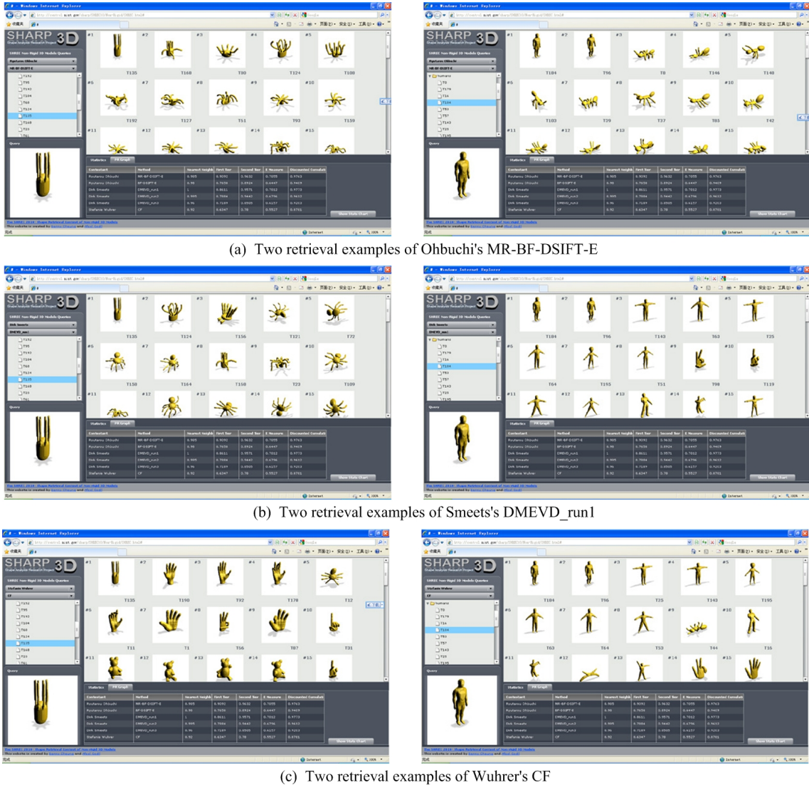
Figure 9: Retrieval examples of three methods using the web interface of the SHREC non-rigid track. The left bottom in the web interface displays the thumbnail of a query and the right top part shows retrieved models.
