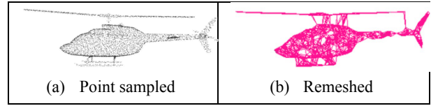
Figure 2. A surface-based 3D model is sampled by oriented points (a) and remeshed (b).
